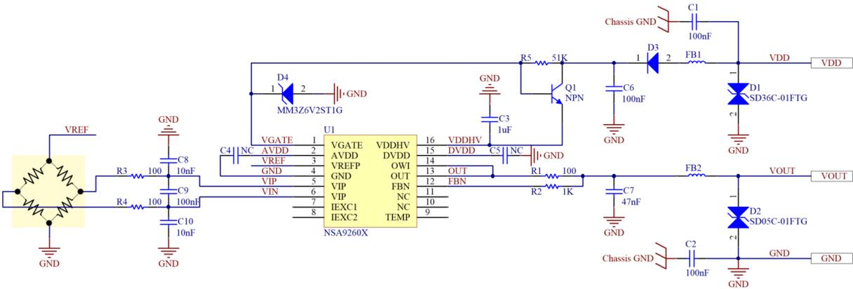
Figure 3.3 Schematic of Analog Voltage Output with High Voltage Input (BJT)
