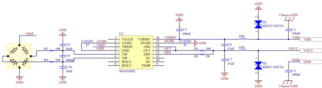
Figure 3.1 Schematic of Analog Voltage Output
