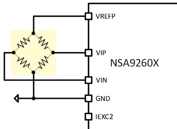
Figure 2.1 Bridge Sensor Using Constant Voltage Source
