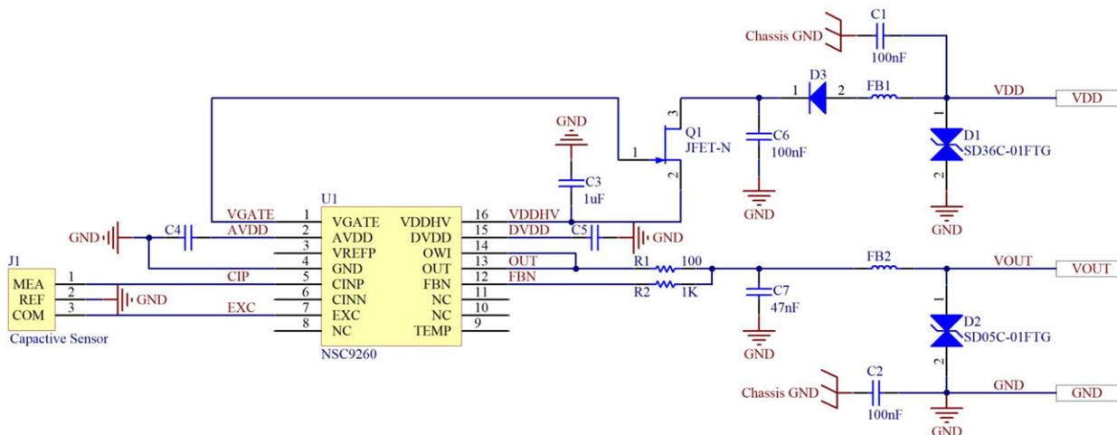
Figure 3.2 Schematic of Analog Voltage Output with High Voltage Input
