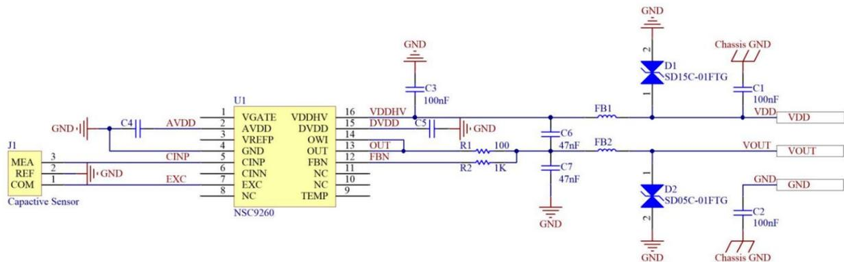
Figure 3.1 Schematic of Analog Voltage Output
