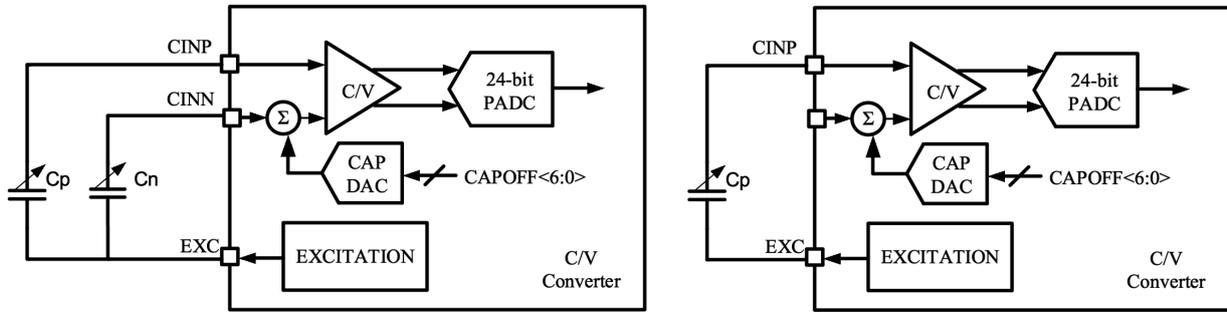
Figure 2.1 Capacitive Sensor Connection Diagram
