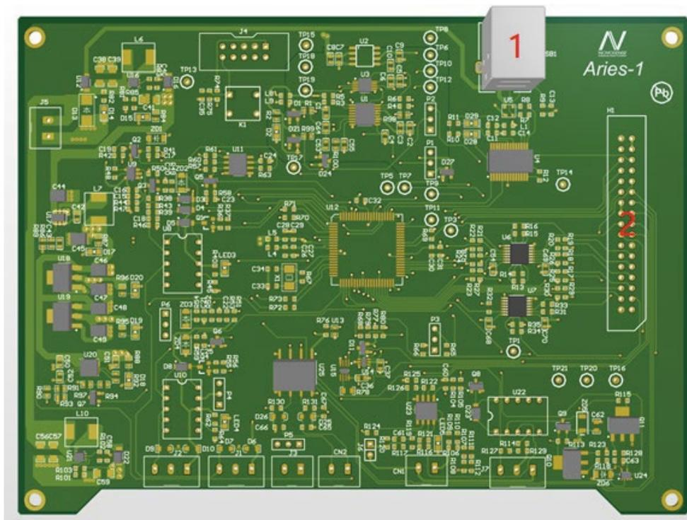
Figure 1. 3D schematic of Controller board
