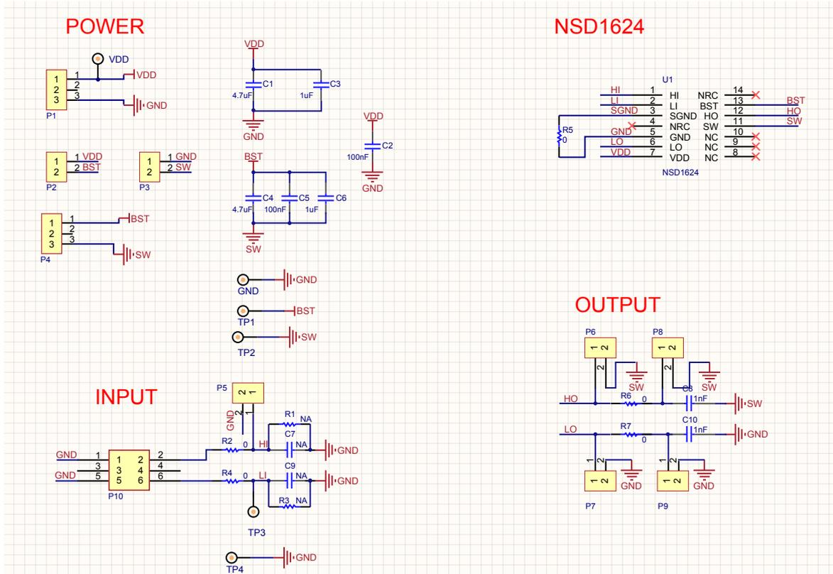
Figure 4. Schematic
