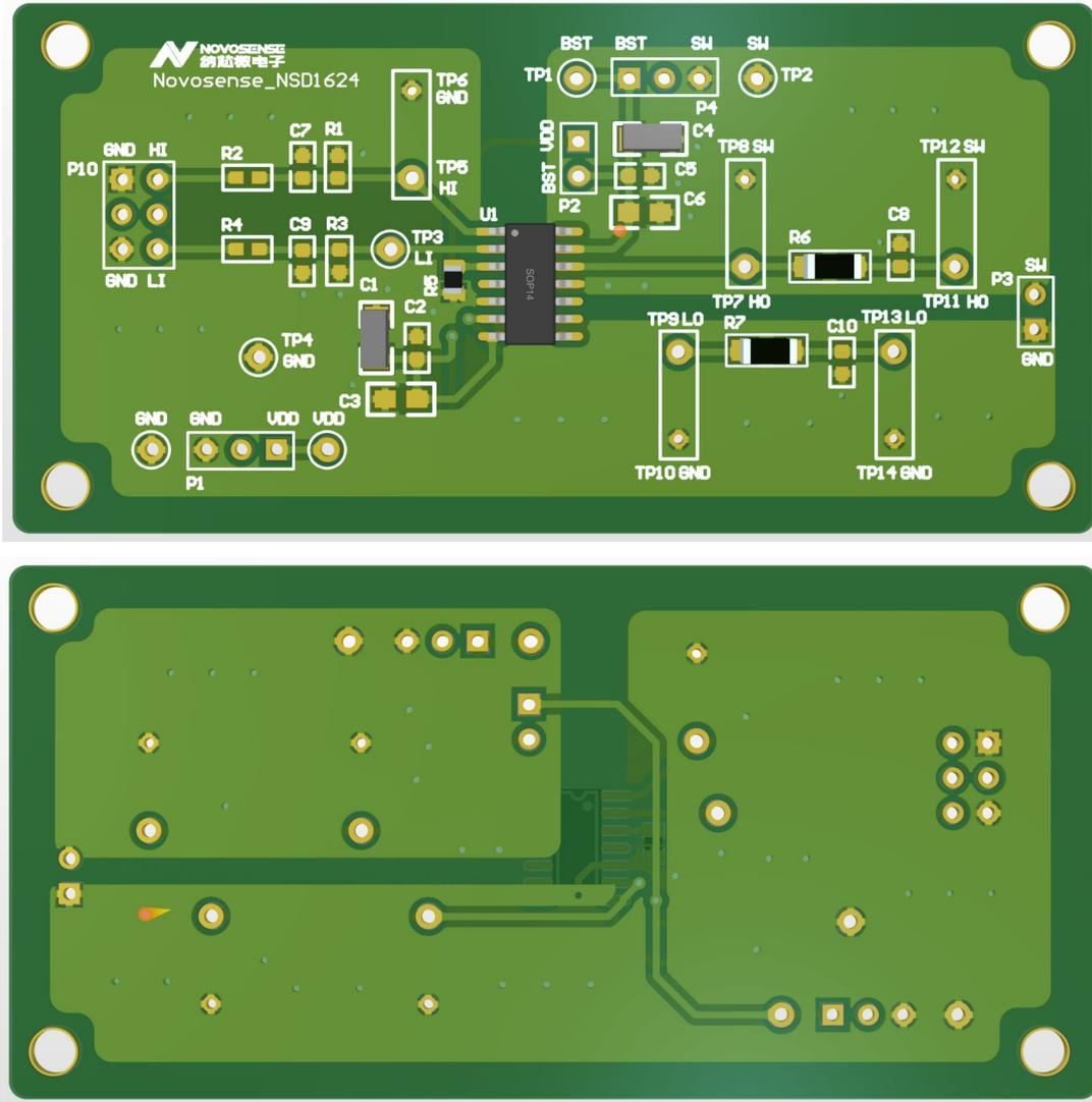
Figure 2. NSD1624-DSPKR Demo Board 3D (Bottom is flipped)
